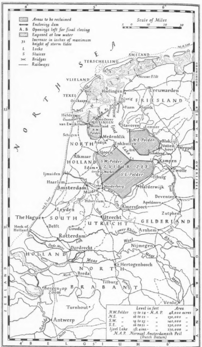
Fig. 2. Sketch-map of the Netherlands showing the plan for the enclosure and partial reclamation of the Zuider Zee
